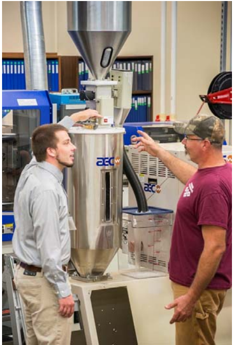
Pelletron's Robert Tausendfreund (left) and Jeff Replogle discuss Sound Technology application of a C20 DeDuster to remove dust from material prior to molding.
