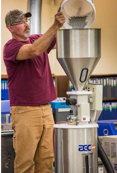
Sound Technology's Jeff Replogle loads material into a dryer with a Pelletron C20 DeDuster located above the dryer hopper.
